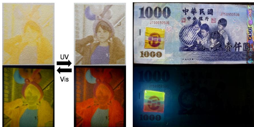
Figure 3: Anticounterfeiting applications based on Pdot RGB inks
