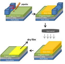
Figure 1:Thin wet film is formed quickly by blade followed by rapid drying to avoid inter-layer dissolution.
